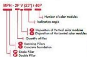
MPH - 2P V (25°) / 40P Single pillar fixed structure with 4 files of horizontal solar modules with 25° of inclination, having 12 solar modules.
