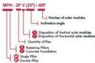
MPH - 4PH (25°) / 12P Single pillar fixed structure with 4 files of horizontal solar modules with 25° of inclination, having 12 solar modules.
